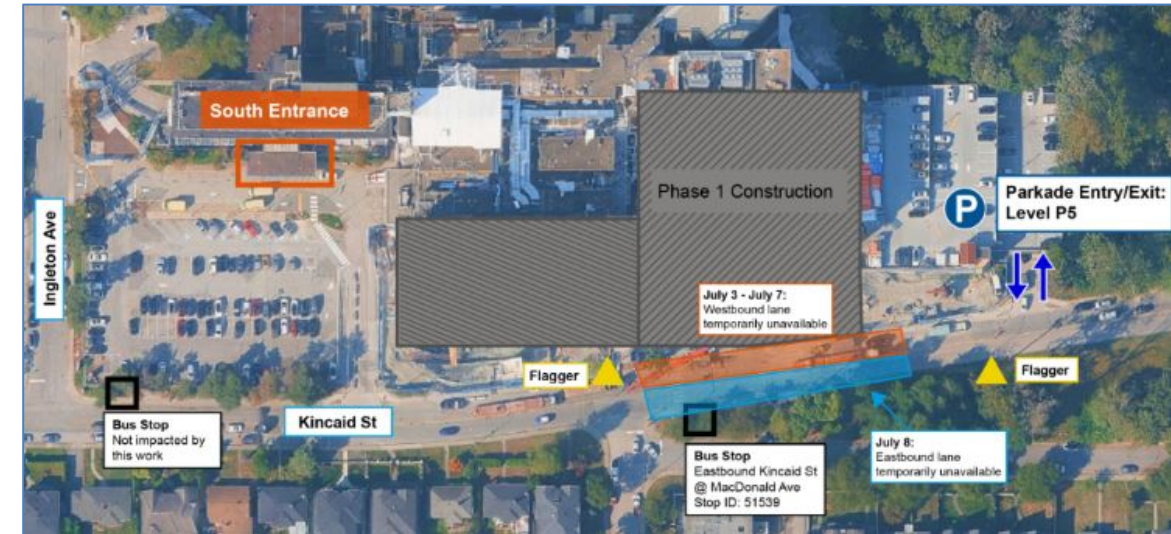
Single lane traffic was implemented along main access road (Kincaid Street) during construction.
