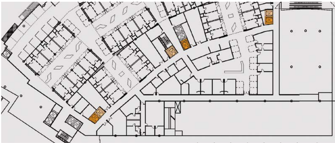
Position of Service Lifts ( Orange )
